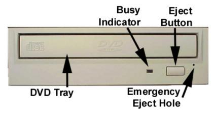
**Loading Tray** Load disc using tray.
